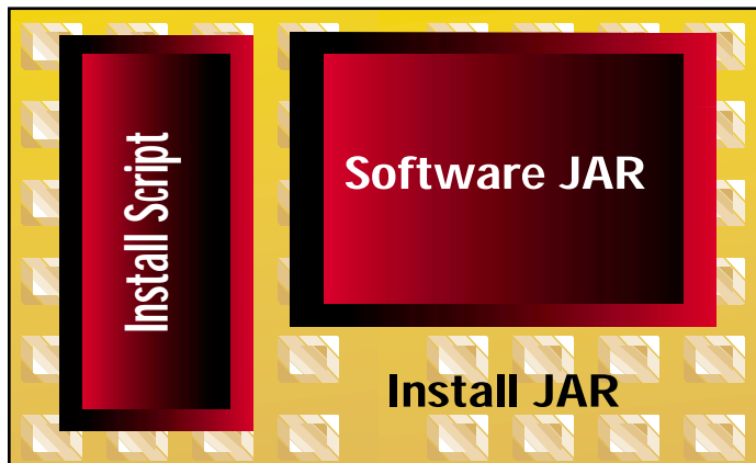
FIGURE 3 Netscape requires your software to be packaged inside another JAR with install script.
